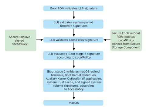
The chip executes code from the Boot ROM in the first step in the chain of trust. macOS secure boot on a Mac with Apple silicon verifies not only the operating system code itself, but also the security policies and even kexts (supported, though not recommended) configured by authorized users.
